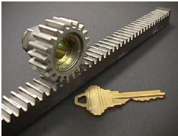
Figure 6: Steel gear and rack cut with an abrasive water jet
